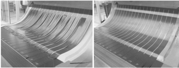
Curved sandwich areas with insufficient and sufficient tack
