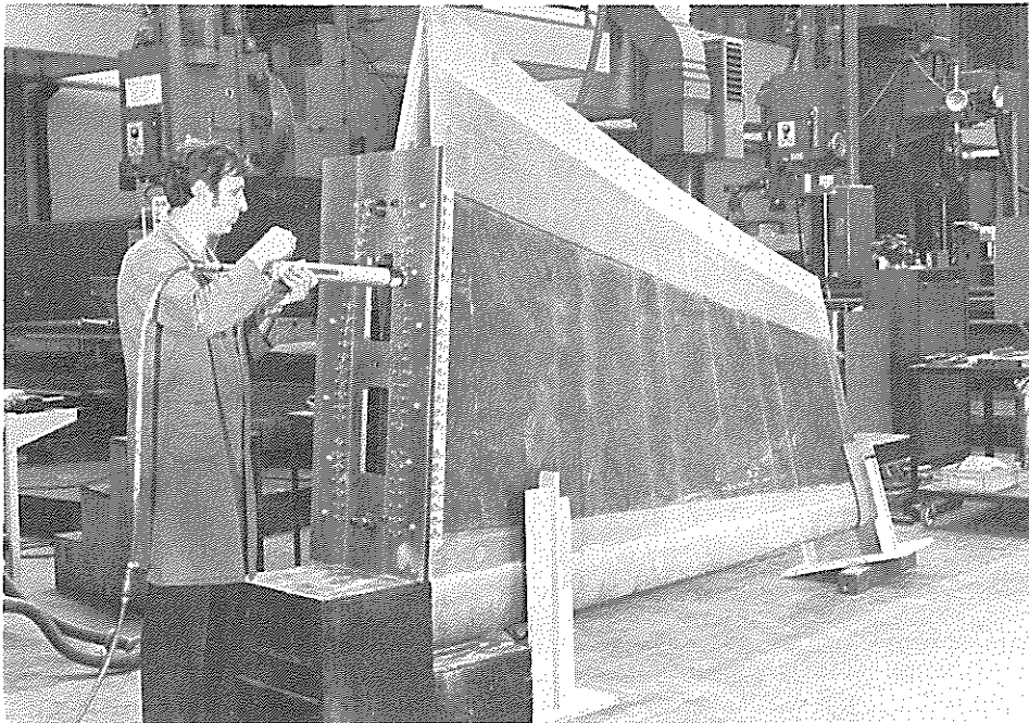
Figure 20: Drilling Process for DNW-Blade
