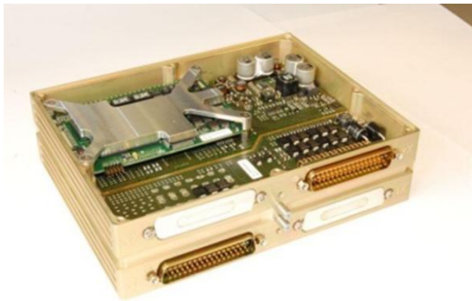
Figure 3: Opened module box of a CPM (manufacturer: SET GmbH, Wangen, Germany).
