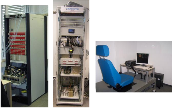
Figure 10: “Core” systems of the verification environment: The middle picture shows the rig (Eurocopter) with FCS modules such as CPMs, IOMs and MR-ACMs as well as real-time test control computer, break-out panels and power supplies. The left picture exhibits the rig (Liebherr) comprising the TR-ACMs and electronic TR-actuator simulation device with break-out facilities. The cockpit station (Eurocopter) with controls and display simulation is shown on the right.
