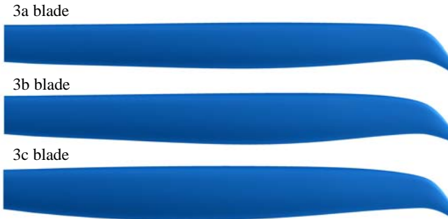
Figure 12: Blade plot of three solutions of the Optimization 3, respectively 3a, 3b and 3c blades.
