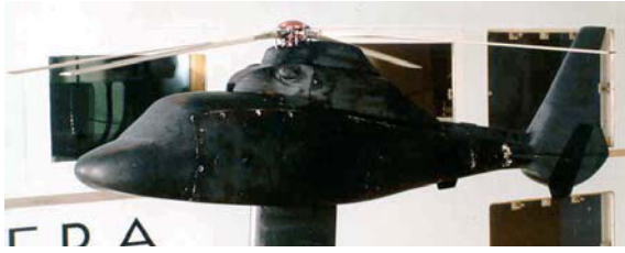
Figure 1 – Dauphin 365N fuselage in ONERA F1 wind tunnel
