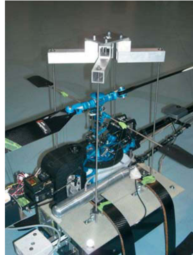
(a) Supporting structure.
