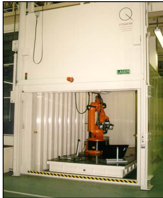
Fig.3: 6-axis industry robot in automatic inspection system of thermal protection parts.
