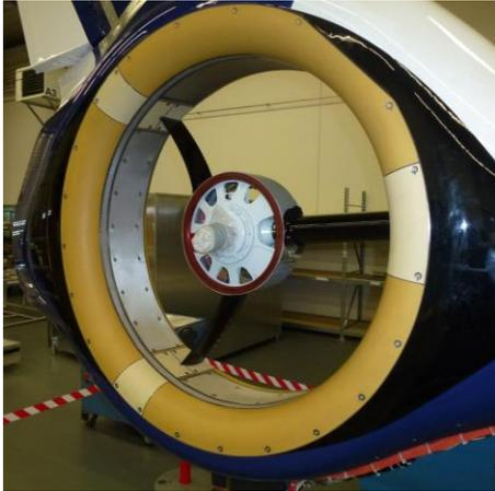
Figure 7: Integrated Fenestron® liner
