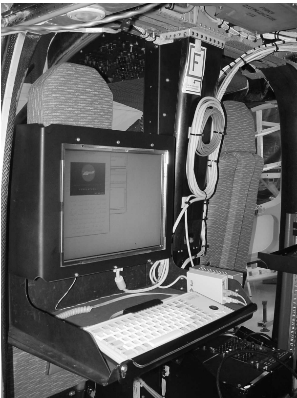
Fig. 8: Operator console in the cargo bay behind the co-pilot's seat.
