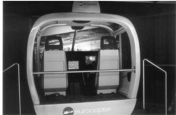
Fig. 6: AWRH simulator featuring a system architecture which is fully compatible with that of the helicopter (hardware and software).
