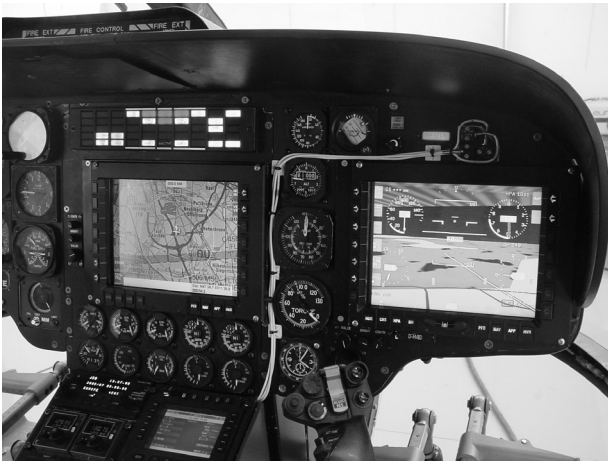
Fig. 4: Pilot Display (PiD, right) and Central Display (CeD, left) in the AWRH testbed.
