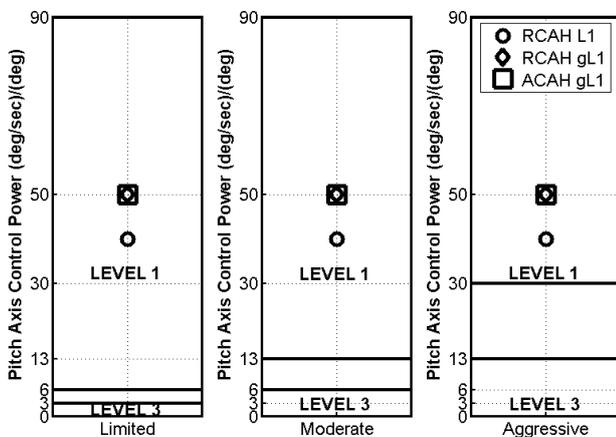
Figure 5. Large amplitude pitch response HQ characteristics
