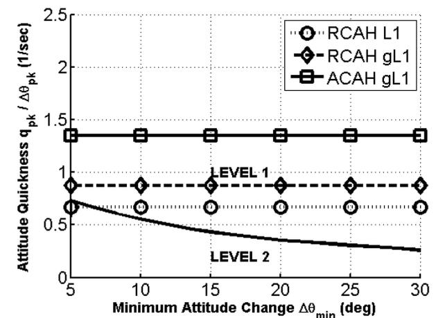
Figure 6. Vehicle dynamics model predicted pitch quickness
