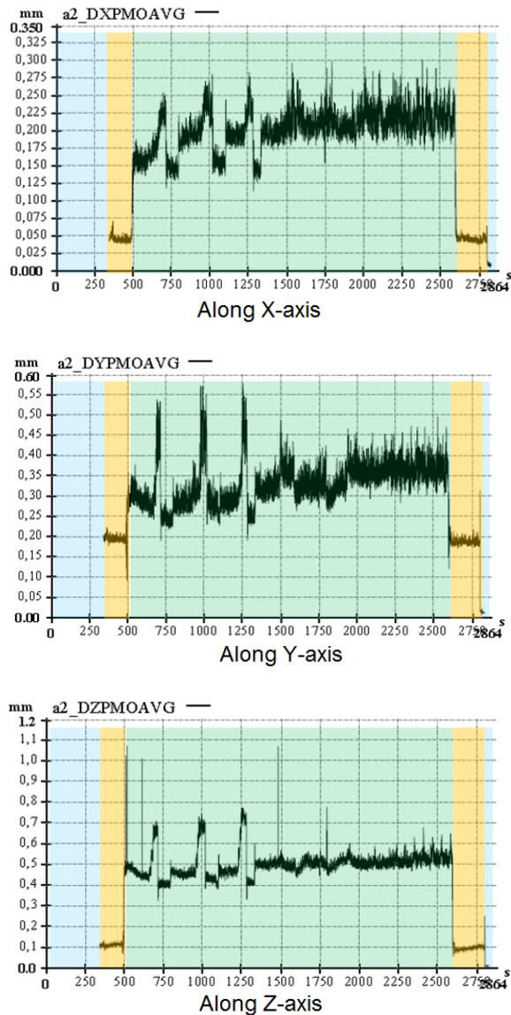
Figure 11: Engine movements (X, Y, Z)
