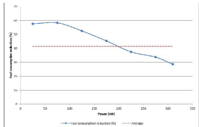
Figure 4: SFC comparison between HCE and turboshaft
