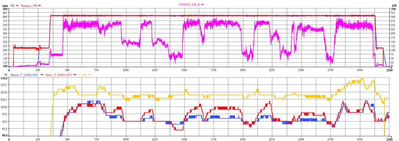
Figure 8: Engine oil and coolant temperatures during a flight at 30°C OAT
