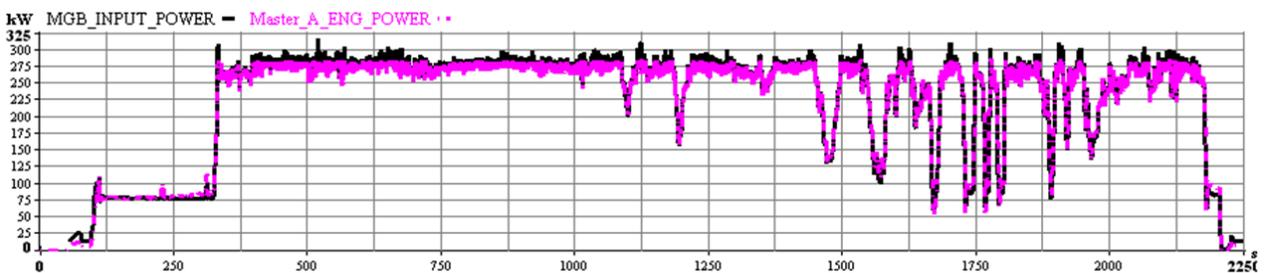
Figure 2: Power output during Maiden Flight
