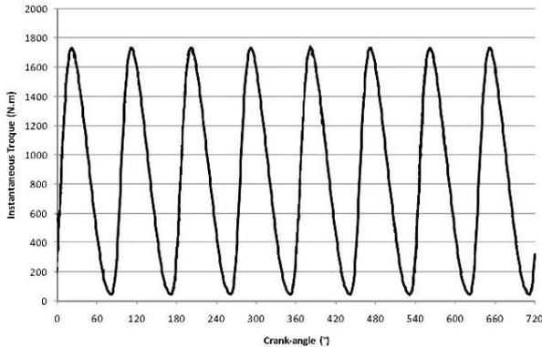
Figure 9: Instantaneous torque at crankshaft
