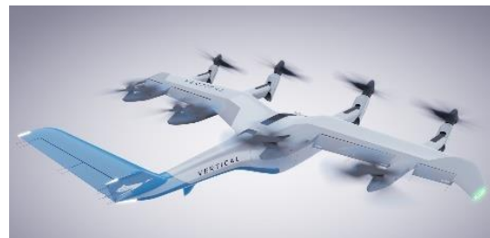
eVTOL (C) : a Lift + Tiltrotor, similar to [18]
