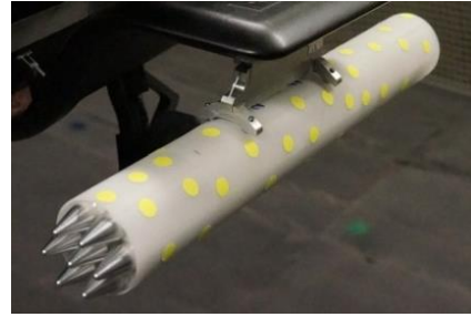
Figure 2. Fully loaded rocket launching store with markers, mounted to the stub wing
