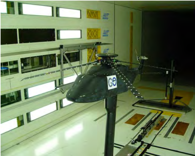
Figure 1: Left: Front view of the GOAHEAD model and experimental setup inside the wind tunnel. Right: Overview of the computational model showing its main components. Wind tunnel section not shown.
