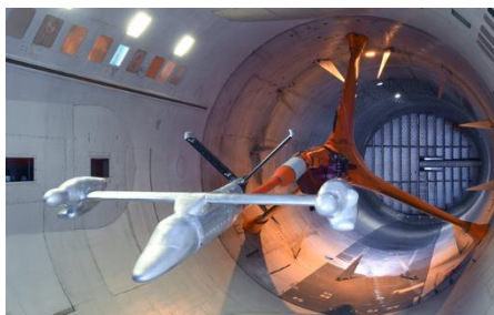
Figure 12 High Speed Wind Tunnel Test in Onera S1MA.
