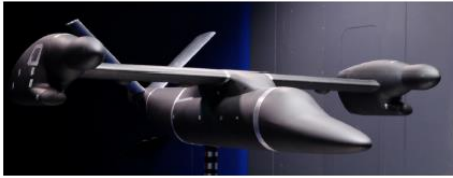
Figure 10 Low Speed Airframe Test in PoliMi WT facility.
