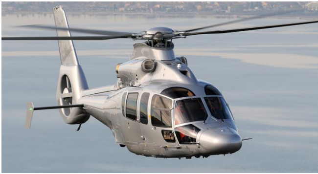
Fig.10: The H155 model that served as a flying test bed for the biplane stabilizer, among other innovations destined for the H160.
