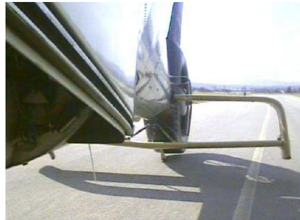
Fig.12: Frame taken from video recording of the left camera that monitors ground clearance around the Fenestron area. The rear guard absorbs the last part of the impact and the Fenestron shroud does not come in contact with the ground.
