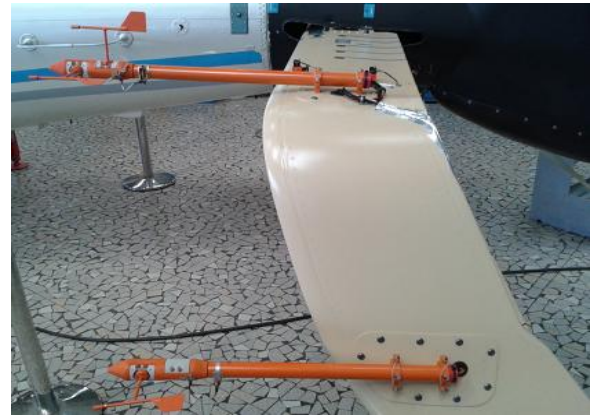
Fig.11: Installation of weathercocks on the outer part of the biplane stabilizer of the H155 flying test bed.
