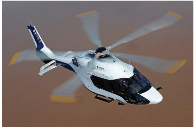
Fig.15: The biplane stabilizer on the H160 prototype during flight testing.
