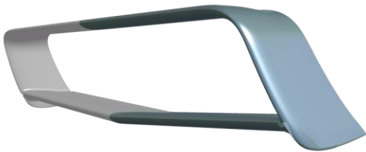
Fig.5: General view of a biplane stabilizer
