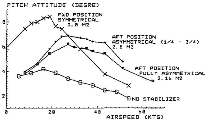
**Figure 6: Wind tunnel determined pitch-up behavior of the NH90 helicopter**
