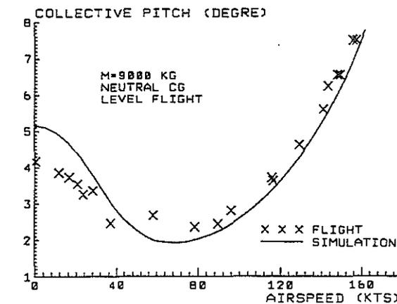
Figure 8: NH90 level flight trim versus airspeed (9000kg, neutral CG, zero sideslip)
