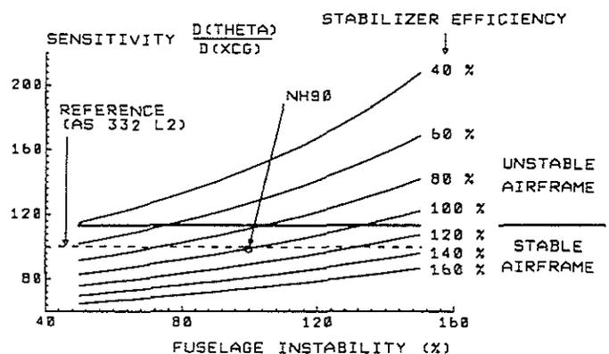
**Figure 4:** Influence of the airframe stability on the attitude sensitivity to CG location
