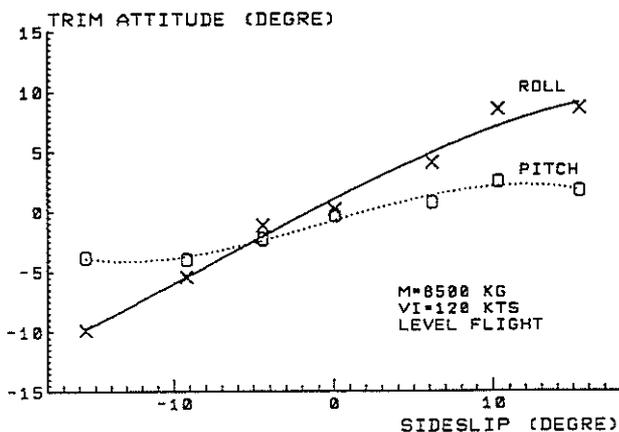
**Figure 10: Sideslip influence (9500kg, neutral CG, 120Kts level flight)**
