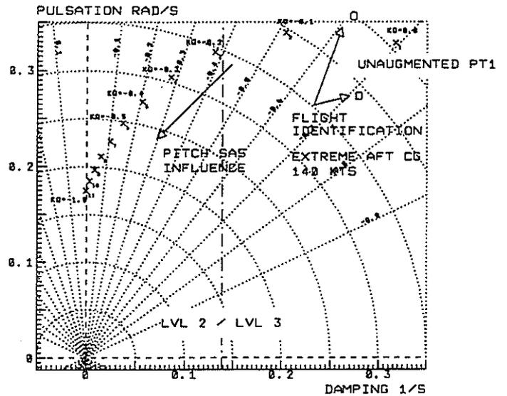
**Figure 11: Prediction of the dynamic stability - adjustment of the basic SAS gain**
