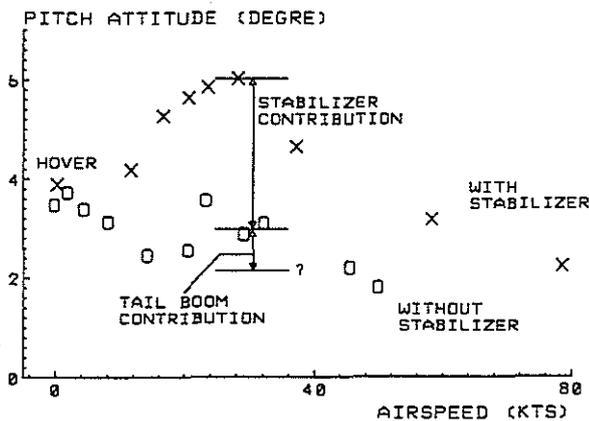
Figure 7: Low speed pitch up: flight test result
