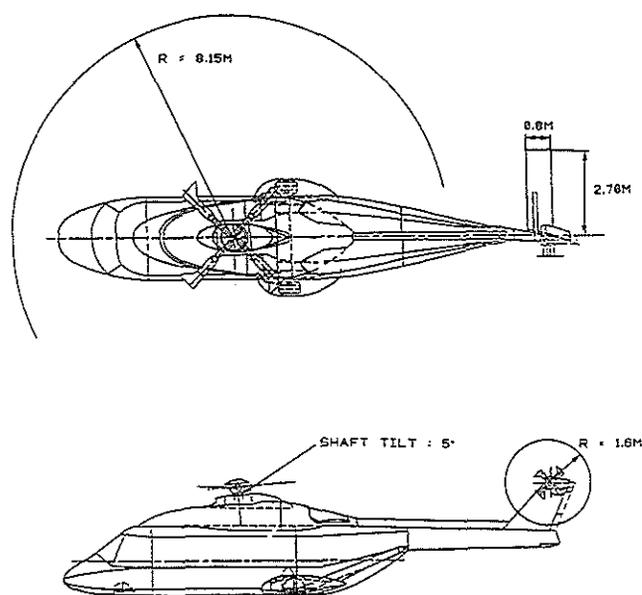
**Figure 2:** NH90 helicopter 3-view drawing
