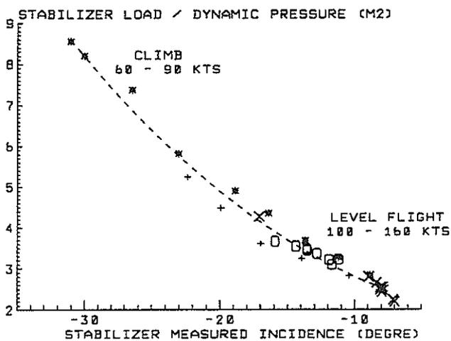
**Figure 12:** measurement of stabilizer load versus local incidence
