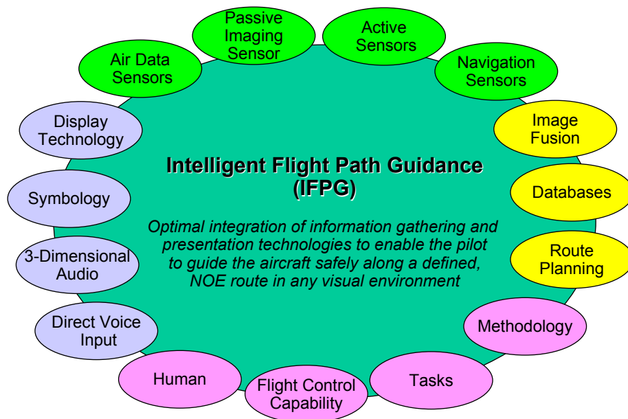
Figure 7: Intelligent Flight Path Guidance components
