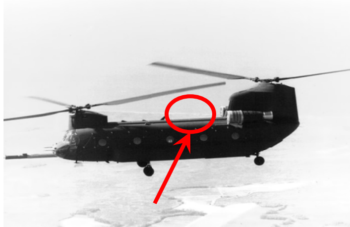
Figure 2: Boeing CH-47D helicopter with an IPS system installed [3].
