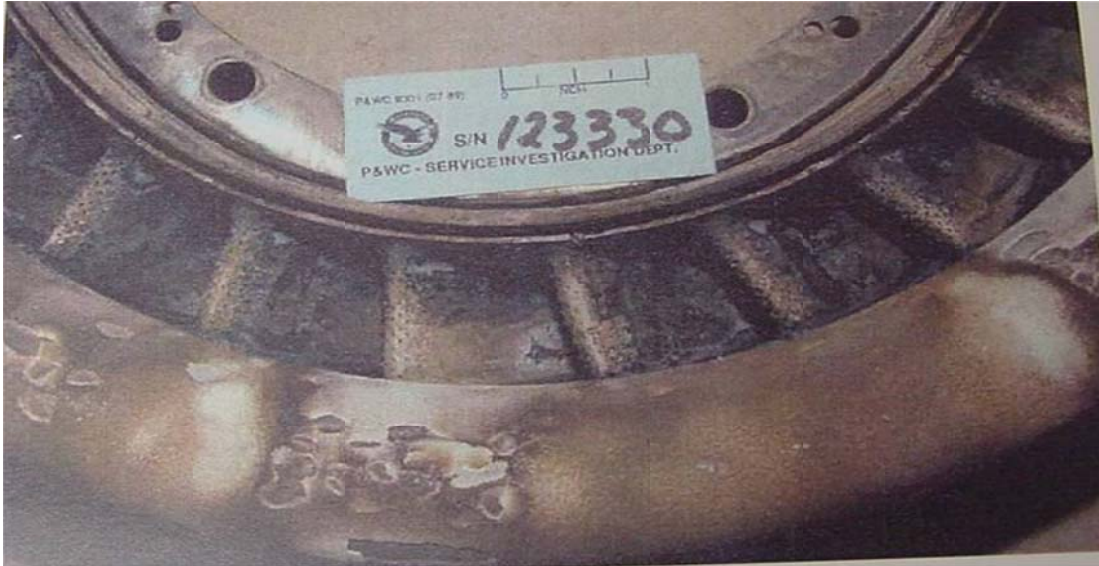
(a) High pressure turbine vanes
