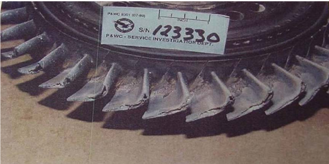
(b) High pressure turbine blades
