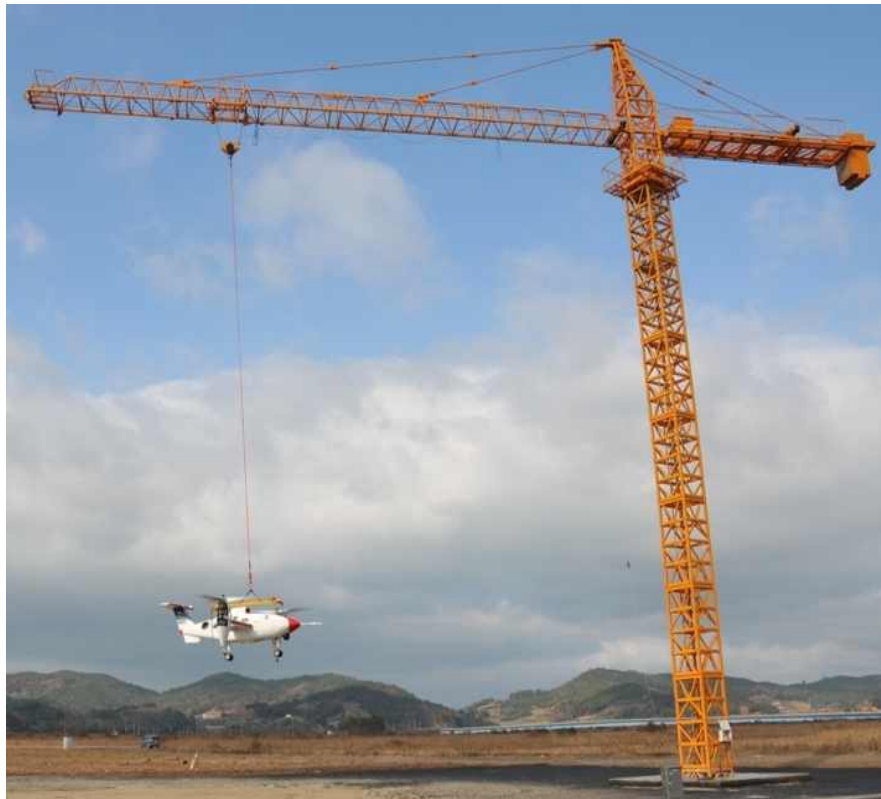
Fig 4 Tether flight test rig for full-scale tiltrotor UAV
