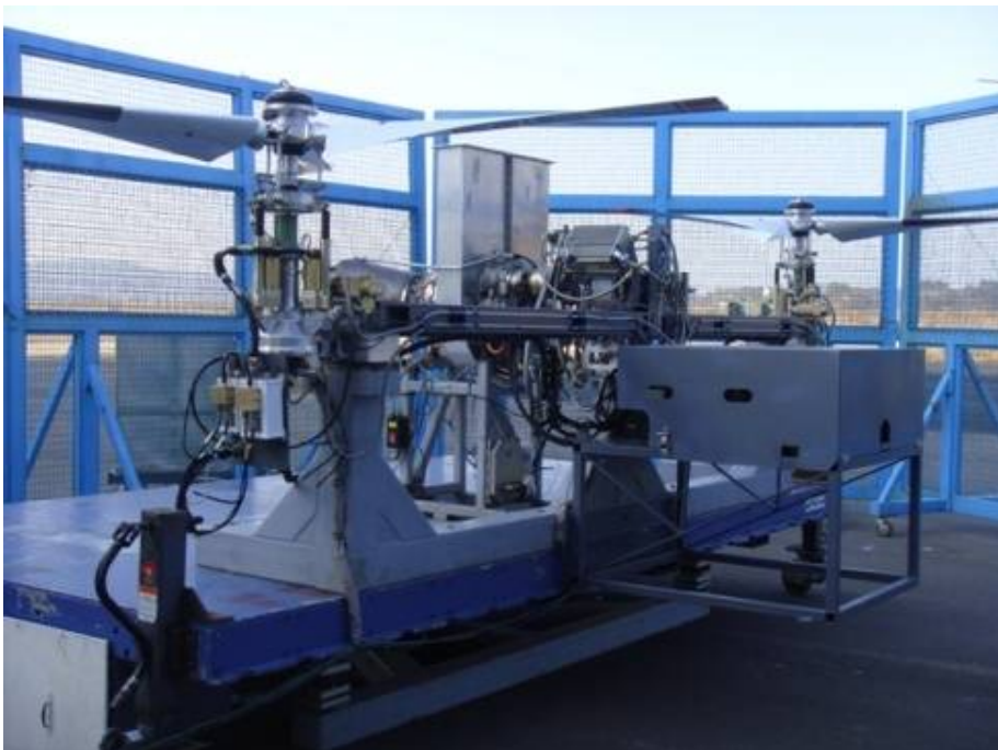
Fig 2 Ironbird test rig for full-scale tiltrotor UAV
