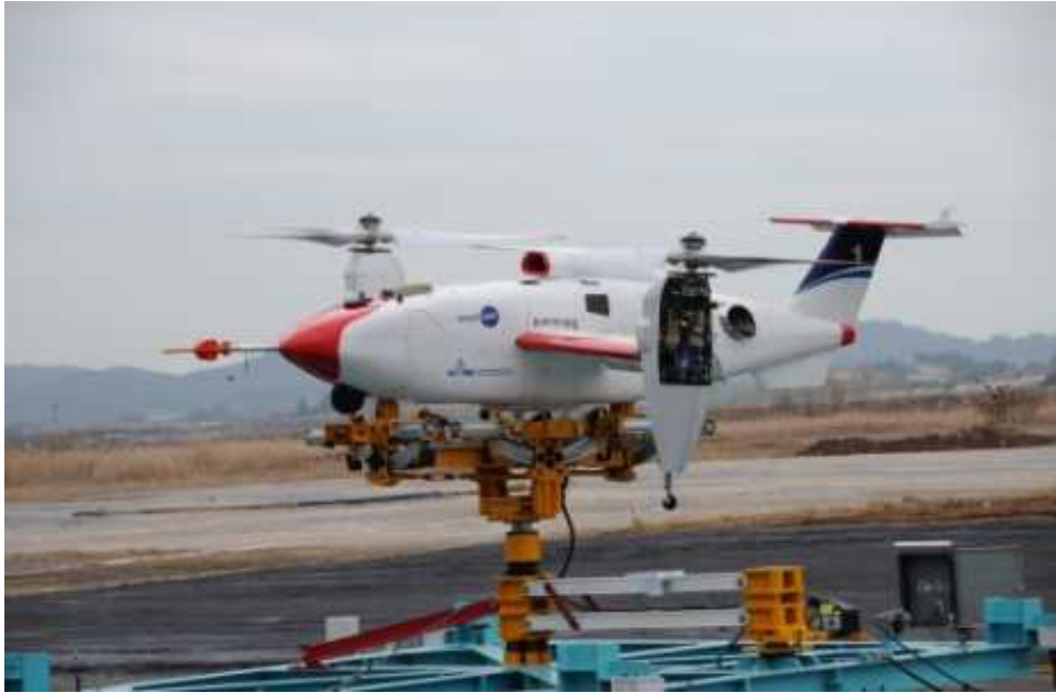
Fig 3 4-degree-of-freedom test rig for for full-scale tiltrotor UAV
