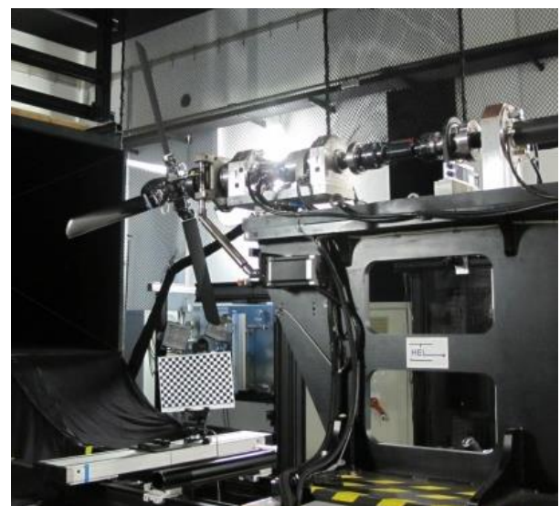
Figure 1: RTG test rig with conventional rotor blades.
