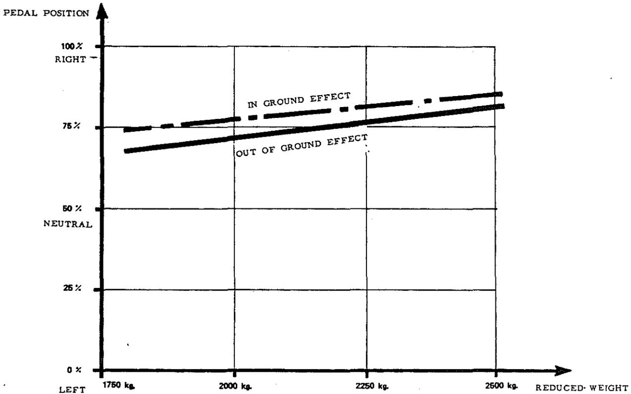
11. PEDAL POSITION IN A HOVER VS. REDUCED WEIGHT
