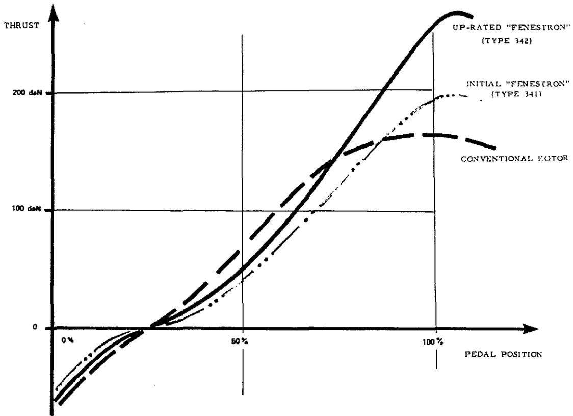
10. COMPARISON OF THRUST PROVIDED BY VARIOUS TYPES OF TAIL ROTOR
