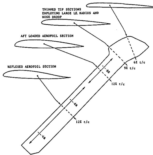
Fig. 18. Lynx/W30 Composite Main Rotor Blade
