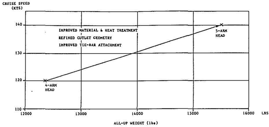
Fig. 17. Potential Improvement in Speed/Weight Capability of Main Rotor Head
