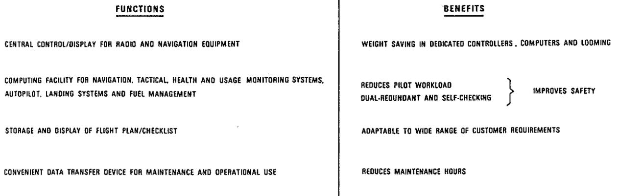
Fig. 26. Digital Core Avionics System (DCAS) for Westland 30
