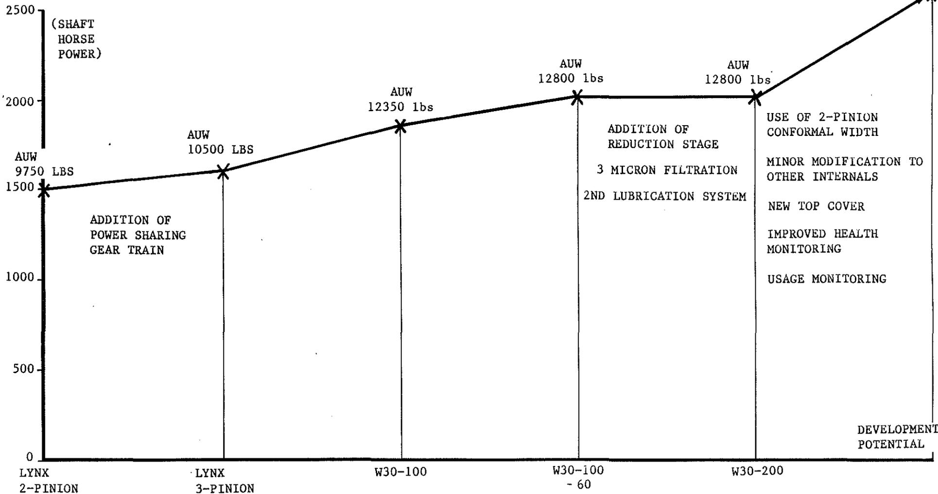
Fig. 15. Development of Lynx/W30 Main Gearbox
