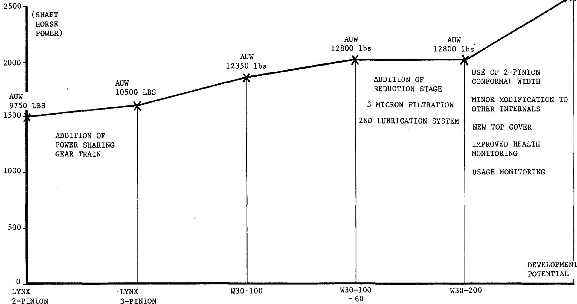
Fig. 15. Development of Lynx/W30 Main Gearbox
