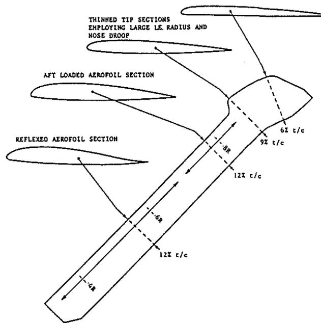
Fig. 18. Lynx/W30 Composite Main Rotor Blade
