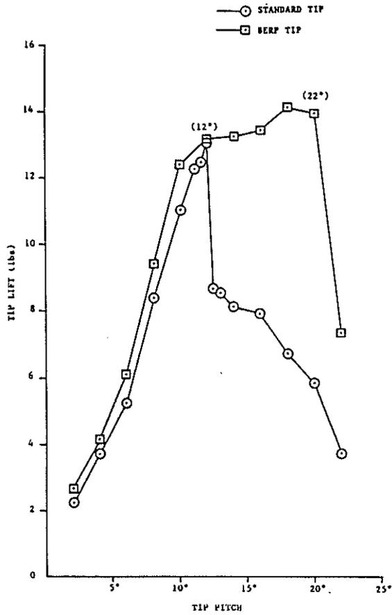
Fig. 20. W30 Composite Blade: Delay of Stall on a BERP Tip
