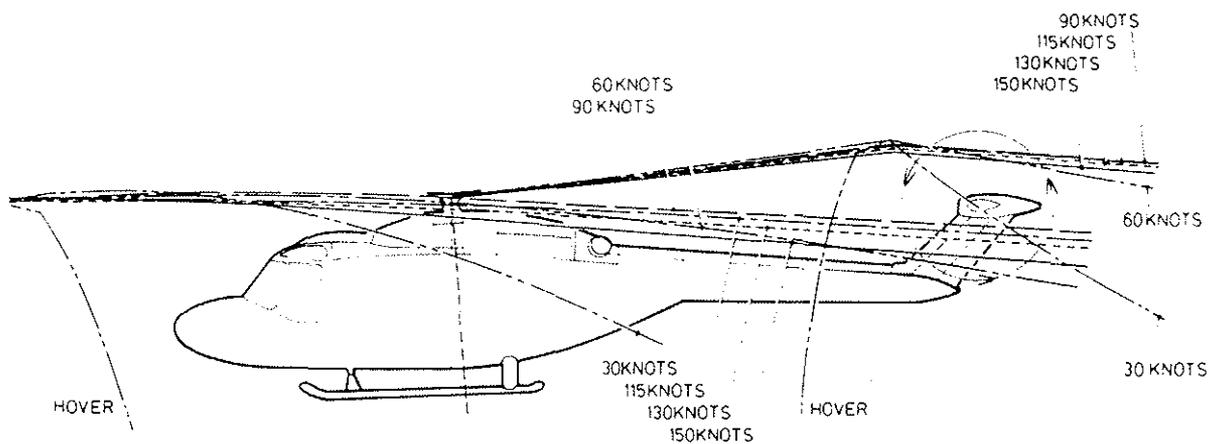
FIG. 6. MAIN ROTOR TIP VORTEX TRAJECTORIES DURING HOVER AND FORWARD FLIGHT
