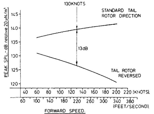
FIG. 9. VARIATION OF IMPULSE PEAK SOUND PRESSURE LEVEL WITH FORWARD SPEED
