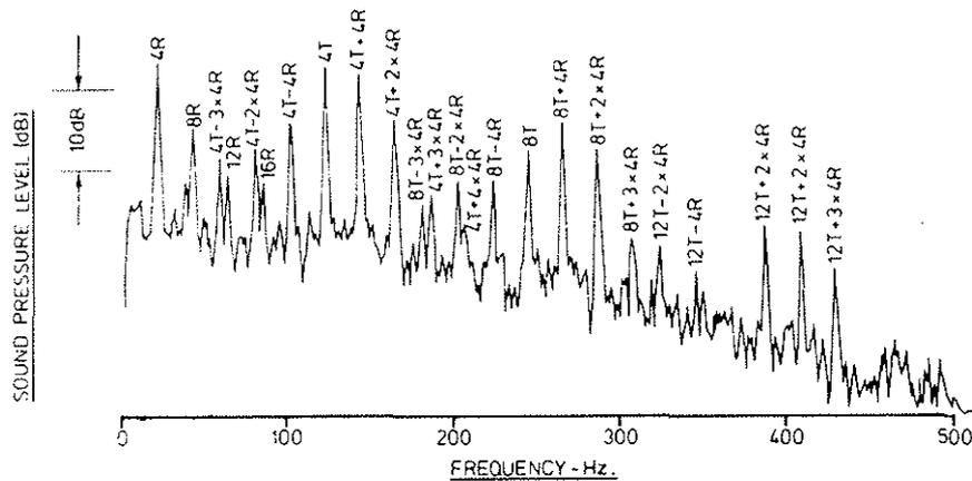
FIG. 2. NARROWBAND ANALYSIS ON REAL TIME ANALYSER - SIGNAL FILTERED AT 1000 HZ, OCTAVE BAND AND FULL WAVE RECTIFIED.
