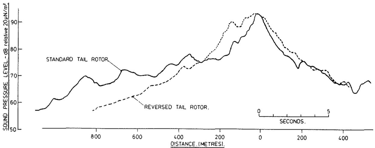
FIG. 11. COMPARISON OF dBA TIME HISTORIES FOR STANDARD AND REVERSED TAIL ROTORS 50 M. ALTITUDE 130 KNOT FLYOVER CONDITION.
