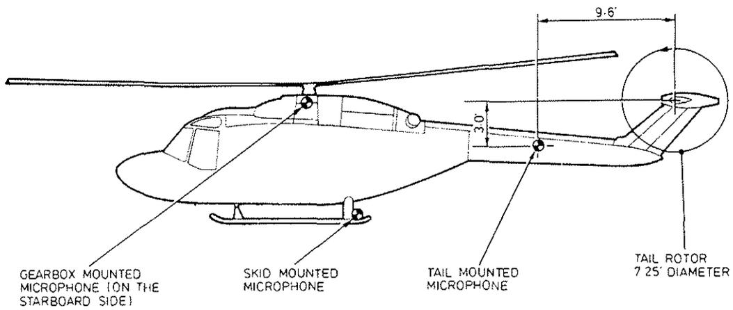
FIG. 1. MICROPHONE POSITIONS ON AIRCRAFT
