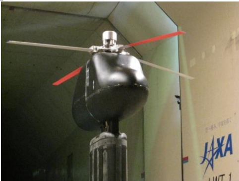
Figure 12. JMRTS(JAXA Multi-purpose Rotor Test System)
