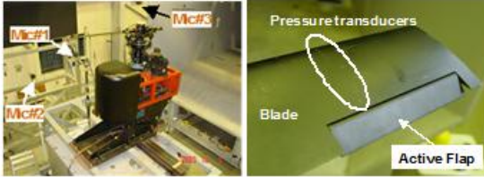
Figure 24. One-blade rotor apparatus in the open section wind tunnel and active flap installation.
