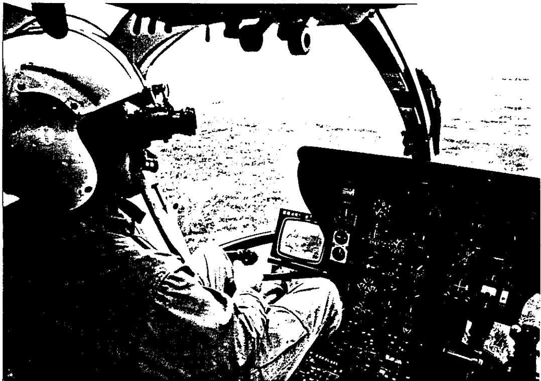
Figure 2 Pilot with helmet-mounted night goggles and Head-down Display in DFVLR Bo 105.
