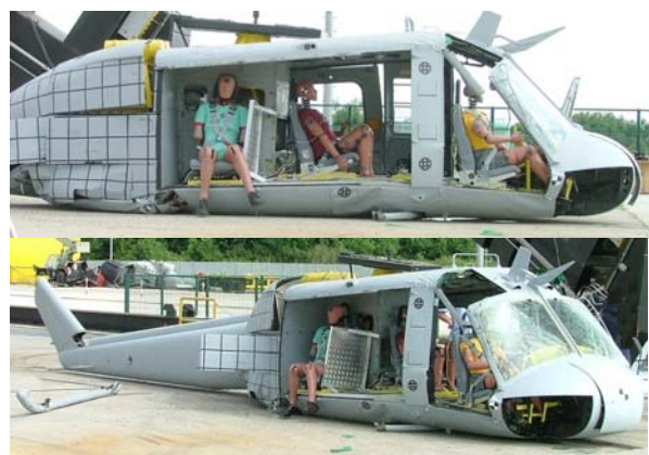
Fig. 4: Bell UH-1D after drop test #1.
