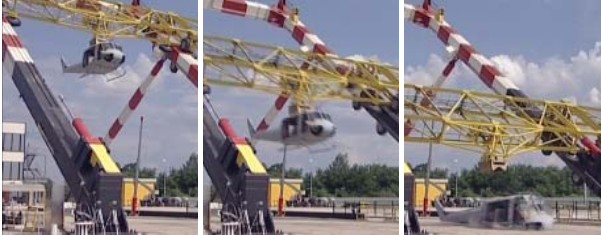
Fig. 1: First HeliSafe TA drop test at CIRA.
