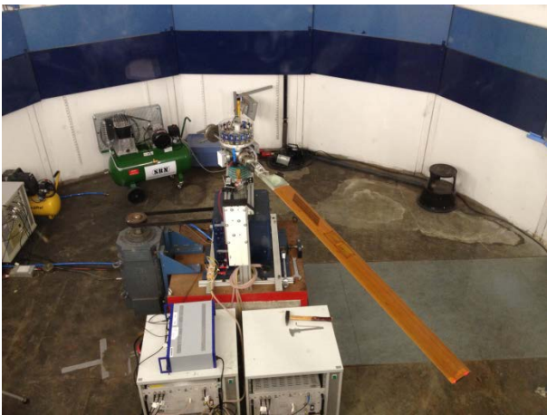
Figure 8: Blade mounted in the test rig
