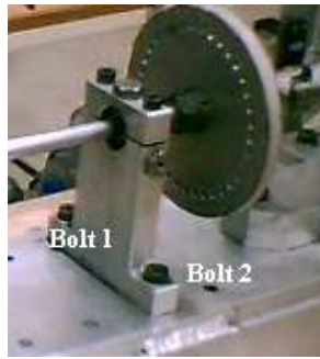
Figure 8: Bearing housing and its base mount
