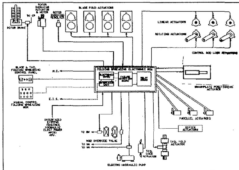
Fig. 1 Folding system schematic
