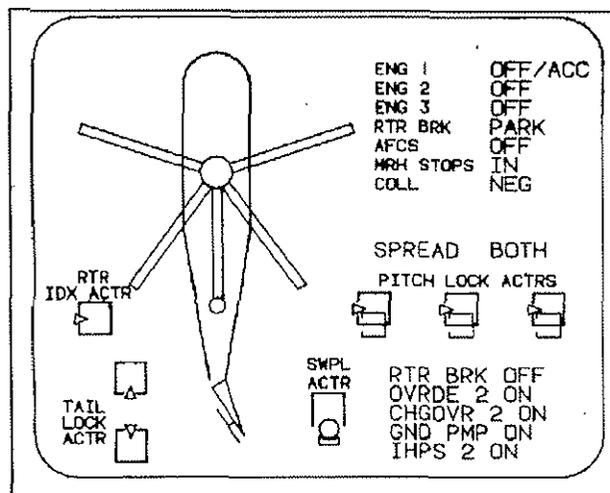
Fig. 5 EIS folding display (example)
