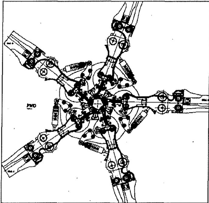
Fig. 6 Main rotor head
