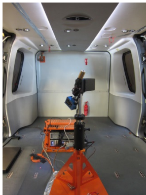
Figure 2: Laser scanning system mounted on the pod
