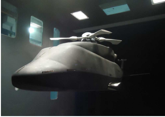
(b) Optimised configuration: small hub-cap, blade stubs fairings, new sponsons, array of VG in the back-door region
