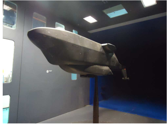
Figure 6: The helicopter model mounted upside-down in the GVPM wind tunnel at POLIMI.
