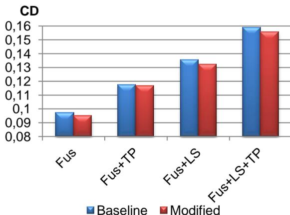
Figure 11. Drag coefficient for different fuselage layouts
