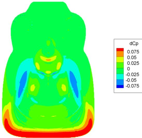
Figure 11. Difference in pressure coefficient distribution between initial and optimized shapes at the rear fuselage
