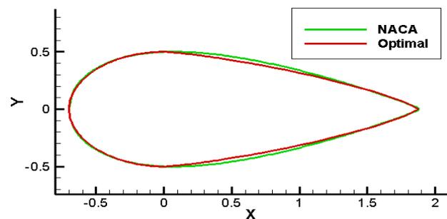
Figure 7. Optimal cross section and aerofoil NACA 00XX
