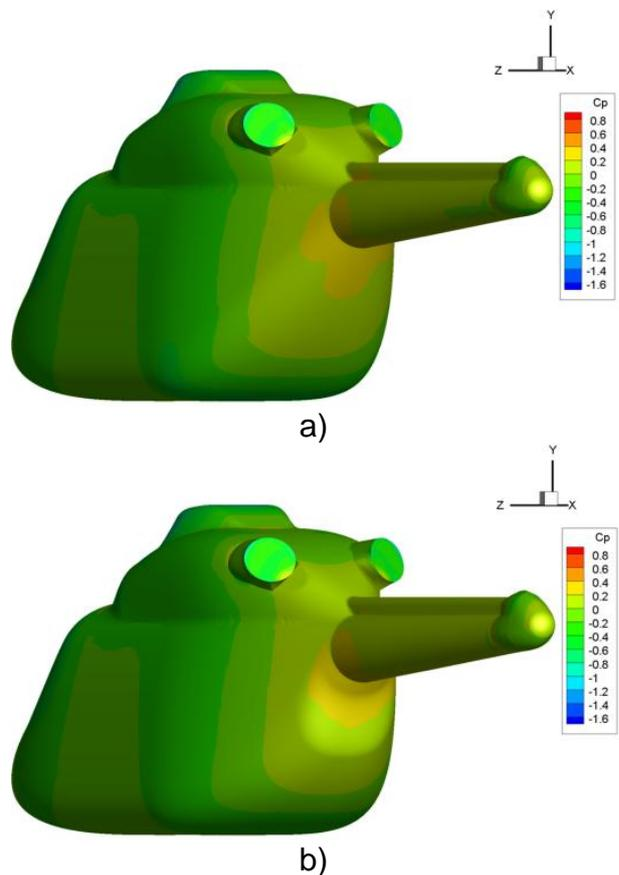
Figure 10. Pressure coefficient distribution: a) baseline; b) modified
