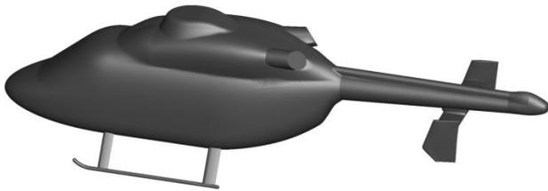
Figure 14. Fuselage layout with modified fuselage and landing fairing
