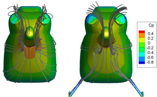
Figure 12. Pressure distribution on the isolated fuselage and fuselage with landing skids
