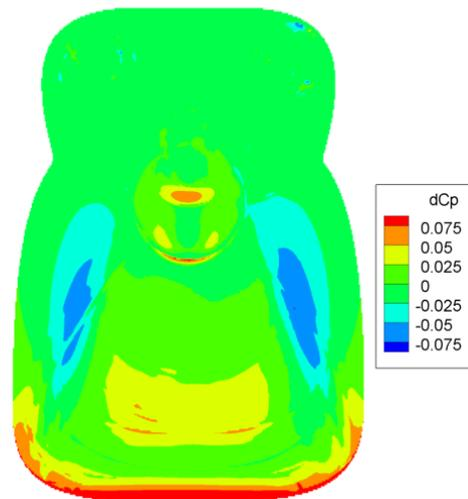
Figure 13. Difference in pressure coefficient distribution between initial and optimized shapes including skids at the rear fuselage
