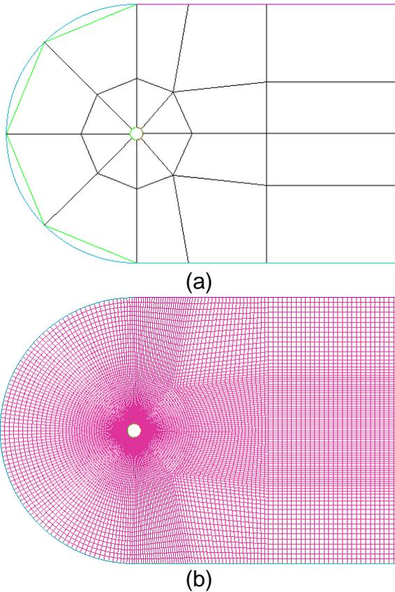
Figure 5. Blocking structure (a) and grid (b) near cross section of landing skids
