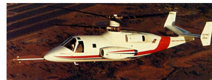
(b) Compound helicopter configuration
