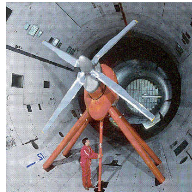
Figure 1 – The Modane test rig and its 90° pitch attitude capabilities (blades of the 7DA1 blades size)
