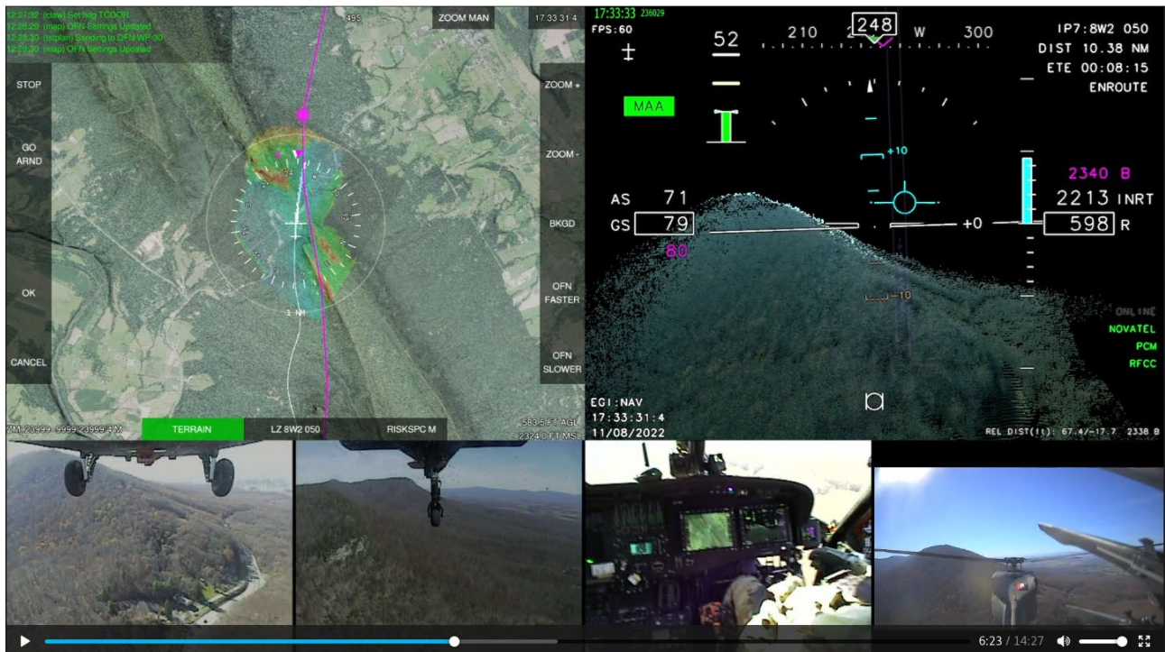
Figure 6: Frame from flight record video. Upper left: pilot's moving map display, shows RiskMinOFN fused terrain in false color overlay with red indicating high terrain and blue indicating low, RAPP route as a magenta line. Upper right: pilot's first-person view display shows true color Lidar data, aircraft state information, flight path vector is a cyan aircraft symbol. Bottom (left to right): forward-facing camera, backward-facing camera, cockpit camera, tail camera.
