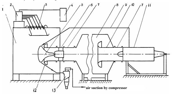
Fig. 17 Tests bench for DPS trials scheme: 1-dusty chamber; 2,3-dust distribution device; 4-dust dosage devise; 5-DPS; 6,7-elongation duct; 8 – receiver; 9-compressed air (scavenge system inject air) conducting line; 10-engine inlet duct; 11-turboshaft engine TV3-117; 12-extracting duct of scavenge air with entrained dust particles; 13-dust collector(dust-air separator).
