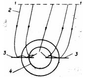
Fig 9. Scheme of particles movement in DPS at partitions presence : 1-plane of initial particles positions; 2-particles trajectories projects; 3-partitions; 4-second stage boundary.
