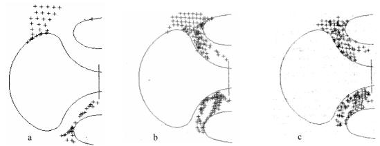
Fig. 5. Distribution of particles ingested in an engine in horizontal plane of DPS symmetry: a - by size 40µ; b - by size 160µ; c - by size 320µ.
