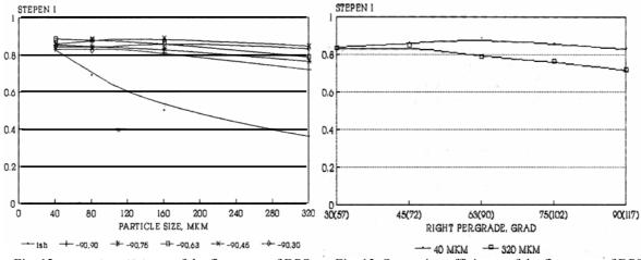
Fig. 12. <u>Separation efficiency</u> of the first stage of DPS versus size of particles at fixed <u>an</u> position of left partition and several positions of right partition. Oblique flow speed is 18 m/s.
