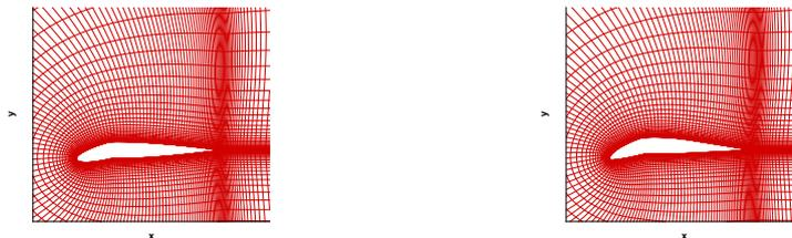
**Figure 3. Body-Fitted Grids for NACA 0012 and VR-7 Airfoils with a Drooped leading Edge**
