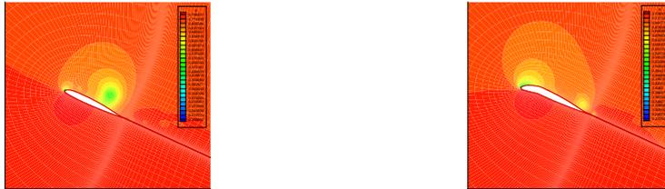
Figure 4. Pressure Field over VR-7 and Ames-01 airfoils with and without Droop at 24.7° Upstroke
