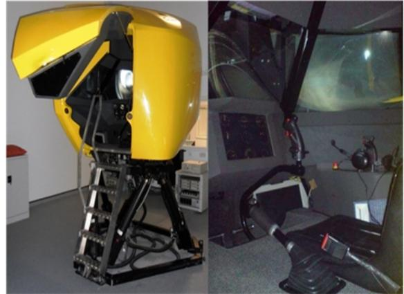
Fig. 17 External and internal views of HELIFLIGHT Research Simulator in the UoL
