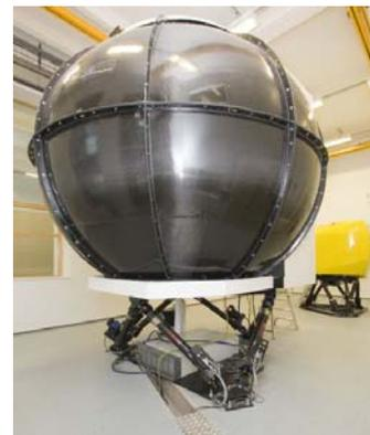
Fig. 10 HELIFLIGHT-R Research Simulator in the UoL [24]
