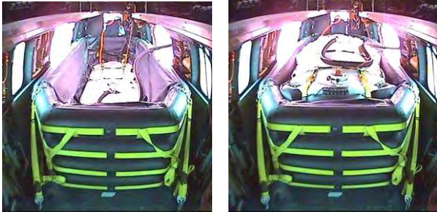
Fig.22 & 23: Water tank kinematic ; Left : empty tank / Right : full tank © Eurocopter
