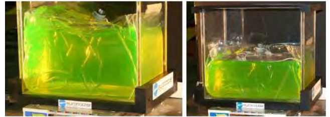
Fig.32 & 33: 50% filled tank. Left : soft tank / Right : soft tank + top plate © Eurocopter
