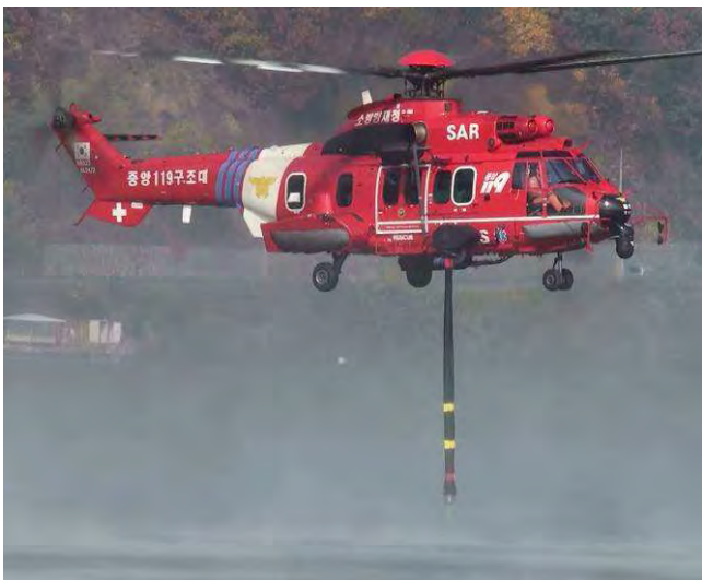
Fig. 28: Ready to dip the pump for refill operation
