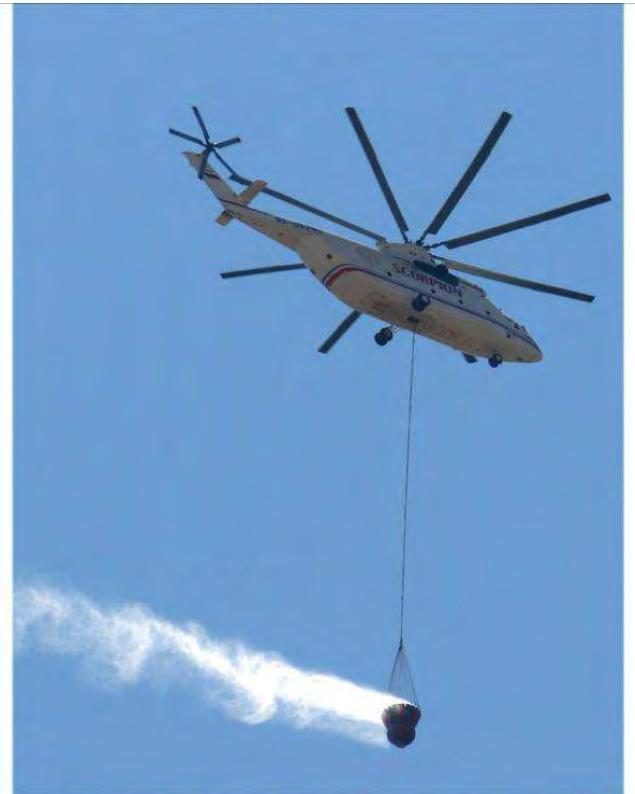
Fig.13: Mi26 carrying a 10t water bucket © Photo KEVREKIDIS 07
