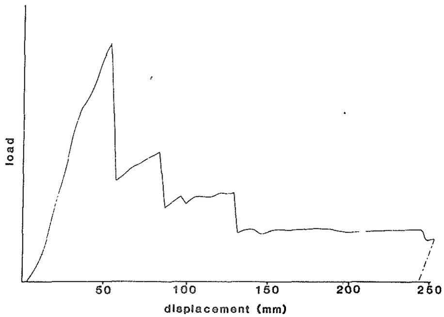
Figure 8. ATF crush test load/displacement curve
