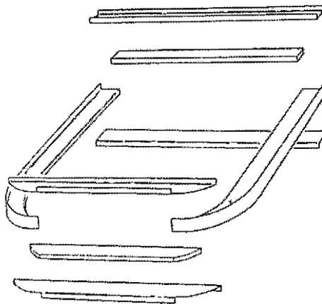
Figure 3. Components of ATF carbon frame
