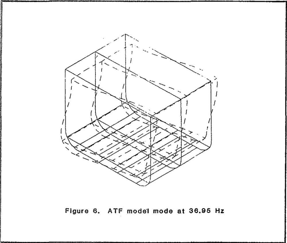
Figure 6. ATF model mode at 36.95 Hz
