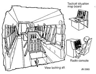
Figure 21. V-22 Command and Control Cabin
