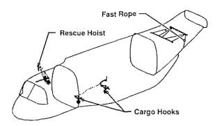
Figure 12. External Load Handling Equipment
