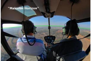
Figure 2 Extended horizon line or Malcolm Horizon (MH) concept
