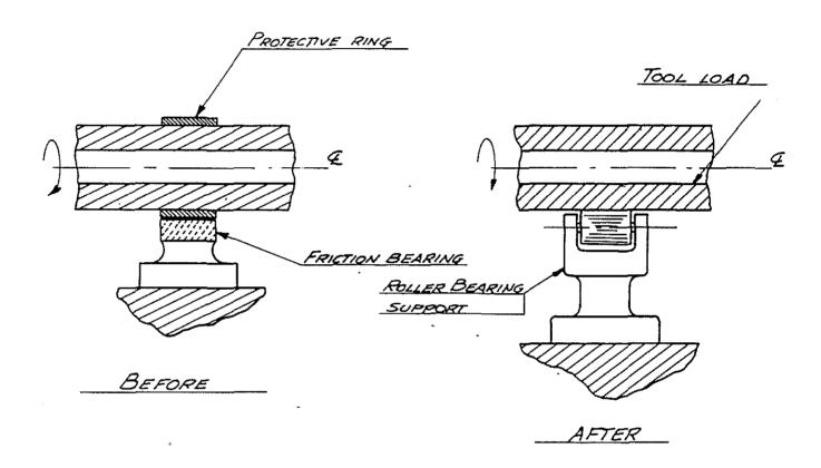
The new roller bearing support, adopted without protective ring, to permit higher cutting speed over hardened the external surface due to tool load.
