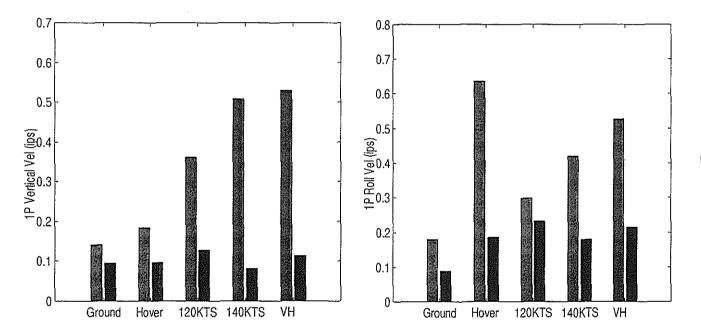
Figure 4. One Pass Optimization of 6 Degrees-of-Freedom Balance (H-60 vertical and roll data)
