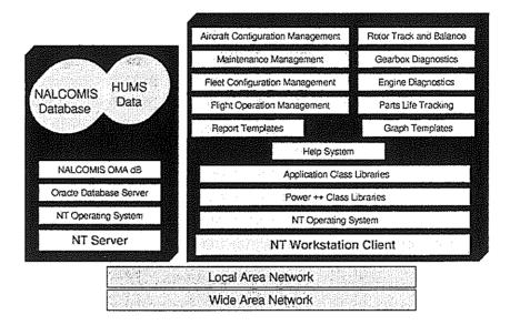
Figure 3. Ground Station Software Integrated With NALCOMIS
