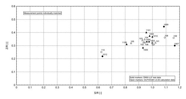
Figure 10 Comparison between OUTWASH (adapted settings) and experimental results
