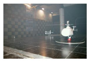
Figure 1 BO 105 model in DNW-LLF test section
