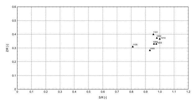
Figure 6 Measured ground vortex core positions in LLS-plane for varied rotor height
