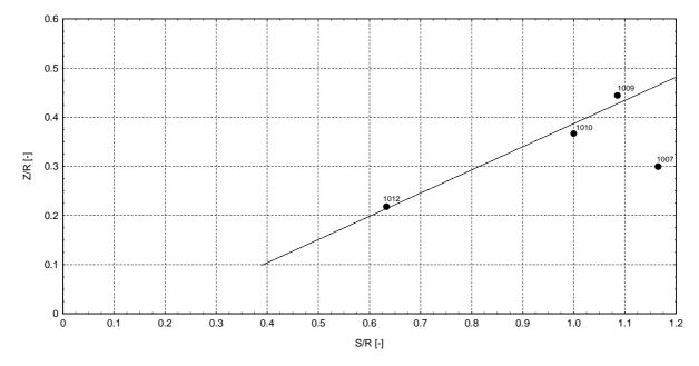
Figure 7 Measured ground vortex core positions in LLS-plane for varied air velocities
