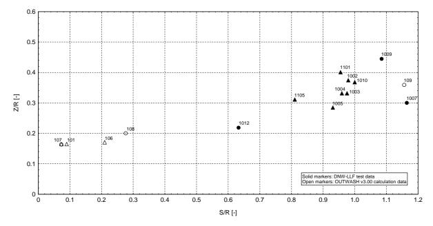
Figure 9 Comparison between OUTWASH (pre-test settings) and experimental results
