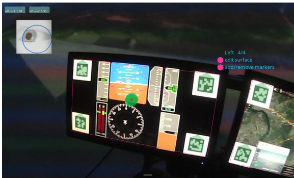
Figure 15: View from eye tracking device camera with estimated gaze focus point and recognised surfaces overlaid on top
