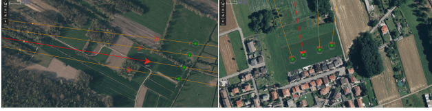
Figure 23: Swarm advancing together (left) and hovering on the destination area (right) as seen from the POS - test campaign 15/11/2023
