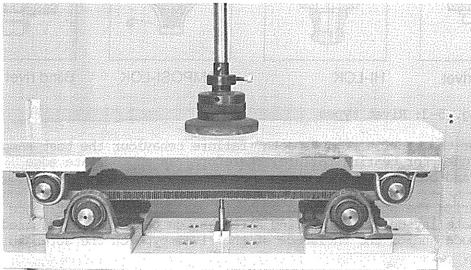
Fig. 5-2: Composite sandwich samples: Bending
