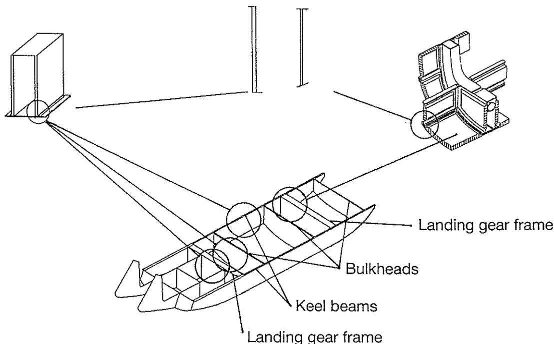
Fig. 6-1: Crash-critical areas of the subfloor structure
