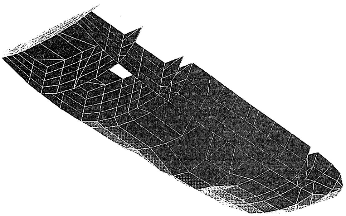
Fig. 3-3: Bottom Panel - Tank loads
