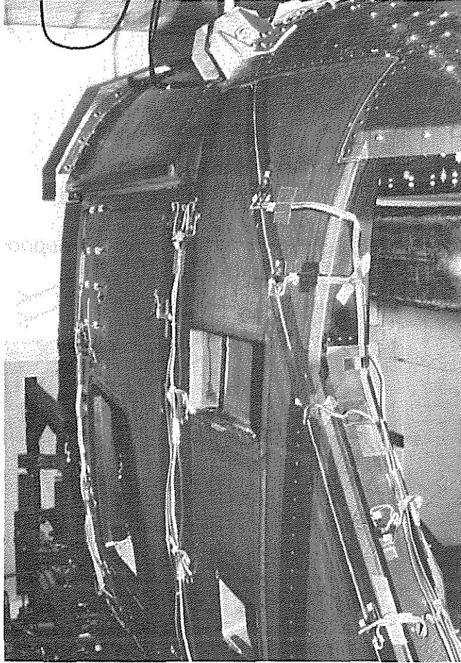
Fig. 5-7: Side panel prepared for load tests
