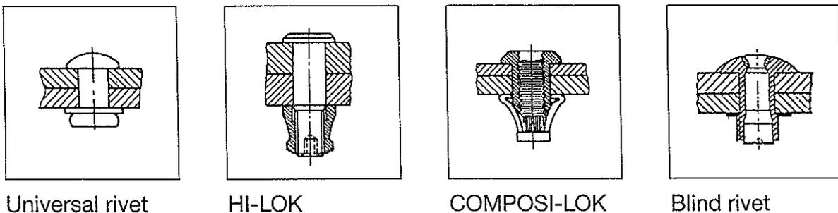
Fig. 5-3: Rivet types
