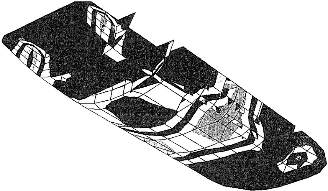
Fig. 3-4: Bottom Panel - Stress Distribution
