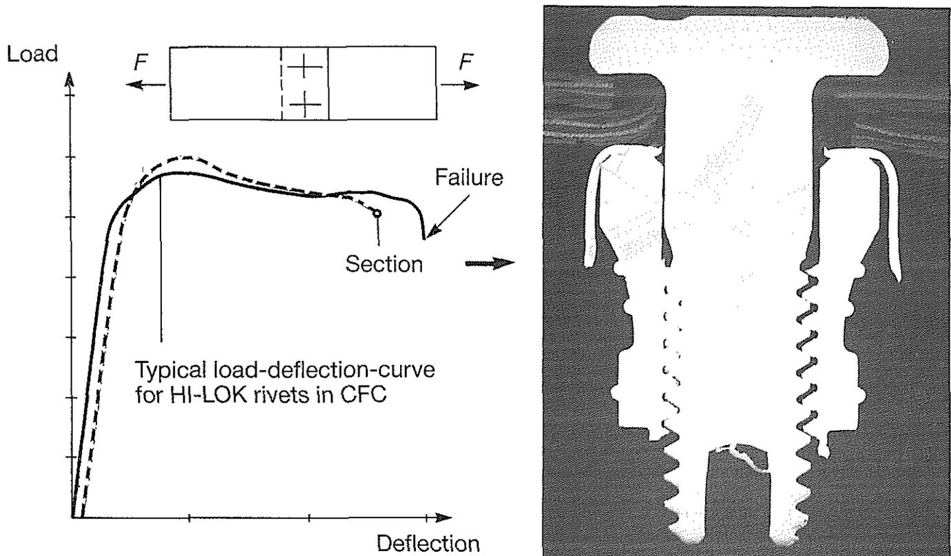
Fig. 5-4: Bearing failure (HI-LOK rivet in CFC)
