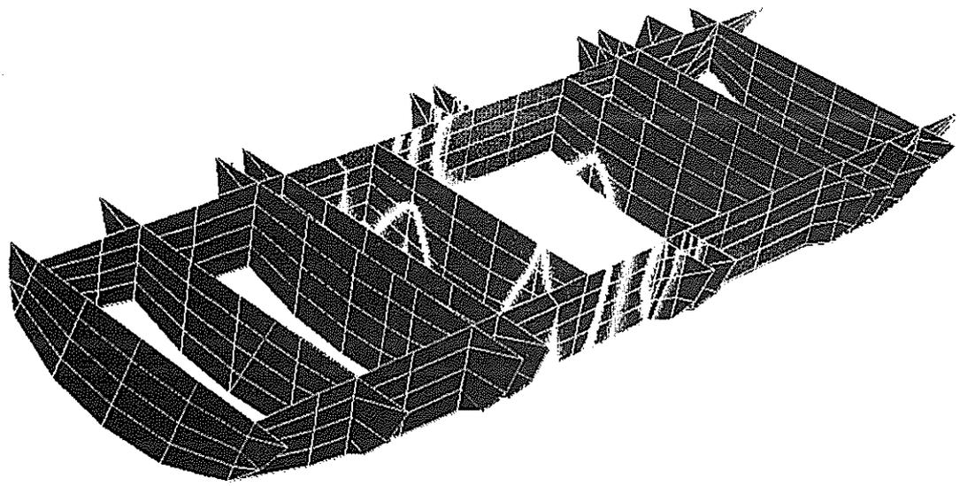
Fig. 3-2: Keel Beams and Spar Elements - Tank loads
