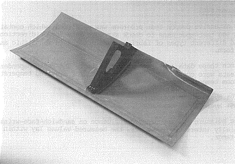
Fig. 4-1: Sandwichpanel bonded to CFC frame
