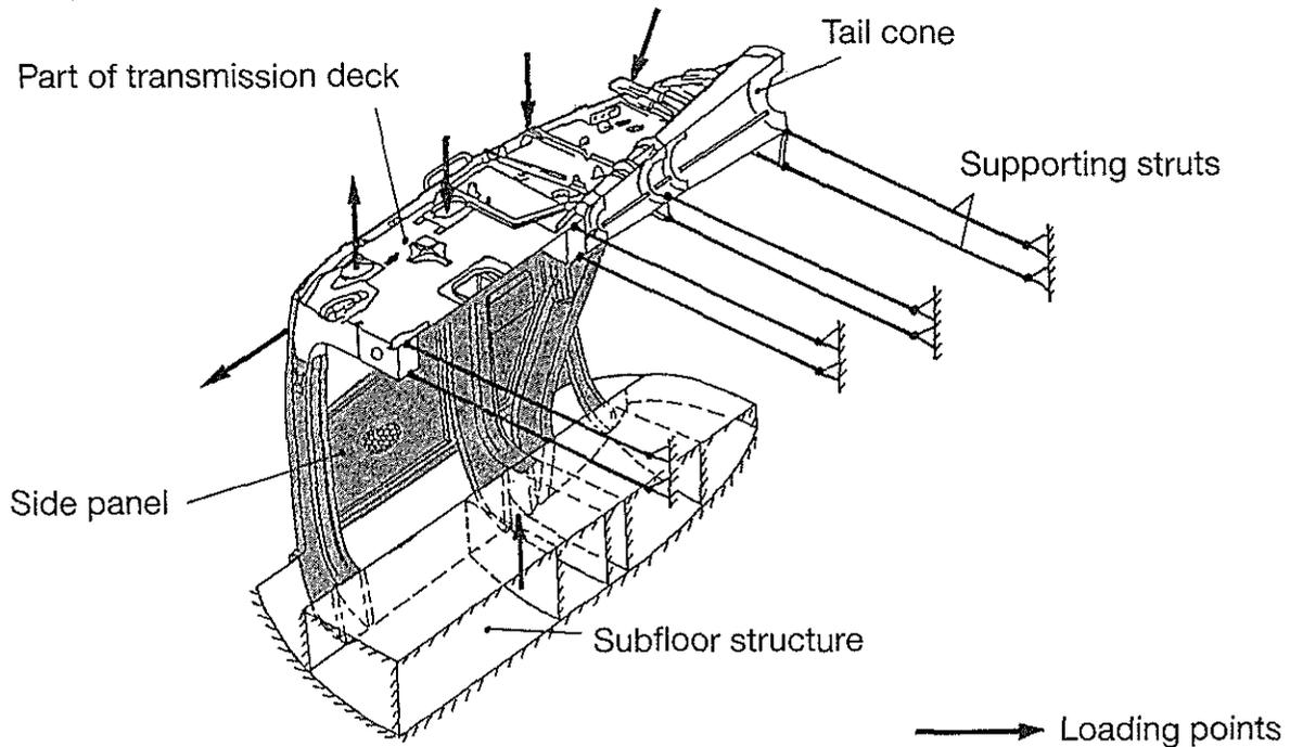
Fig. 5-6: Schematic view of the component test set-up
