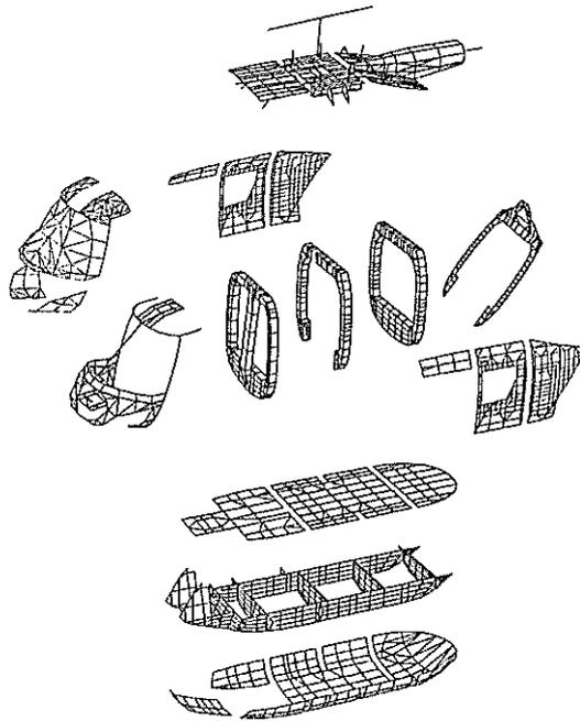
Fig. 3-5: Break down of Finite Element Model
