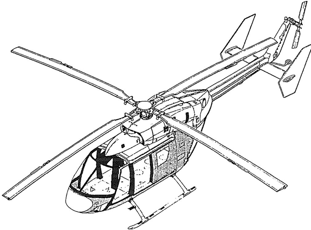
Fig. 1-1: Composite Light Helicopter Fuselage
