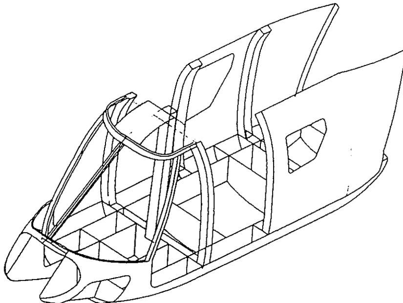
Fig. 2-2: Composite part of the experimental airframe
