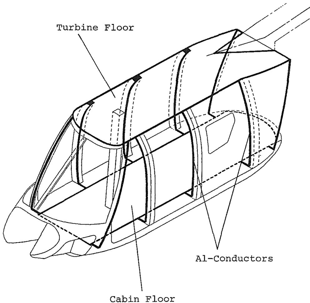
Fig. 2-6: Basic electrical concept
