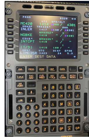
Figure 5. A320's Multi-Function Control and Display Unit. Credits: TXT E-Tech.
