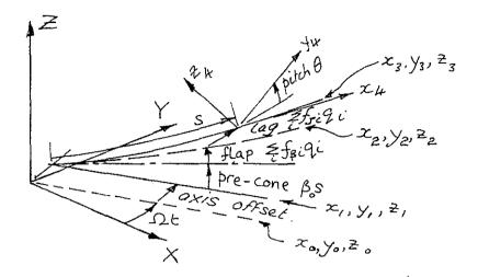
$R = \{x, Y, Z\} - fixed coords \quad r = \{x_4, y_4, Z_4\} - blade coords$   $Fig = 1 - Sets \quad of \quad axes$
